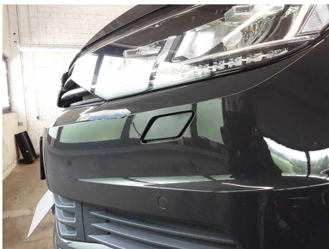
Damage 5: Front bumper: Front strip (Abdeckung) - Damaged - Replace
