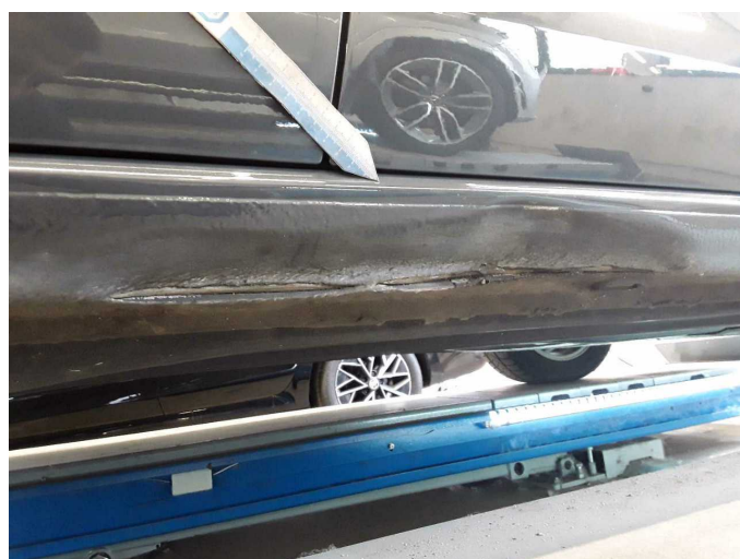
Damage 11: Sill - right side: Sill (Teilersatz) - Deformed - Replace
