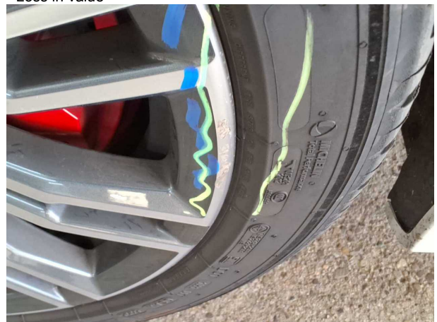
Damage #6: Wheel / tyres: Alloy rim - front left side - Scratched - Loss in value
