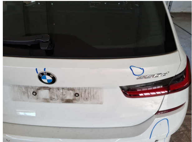
Damage #9: Boot lid / rear door: Boot lid - Dent / paintcoat damage - Smart repair
