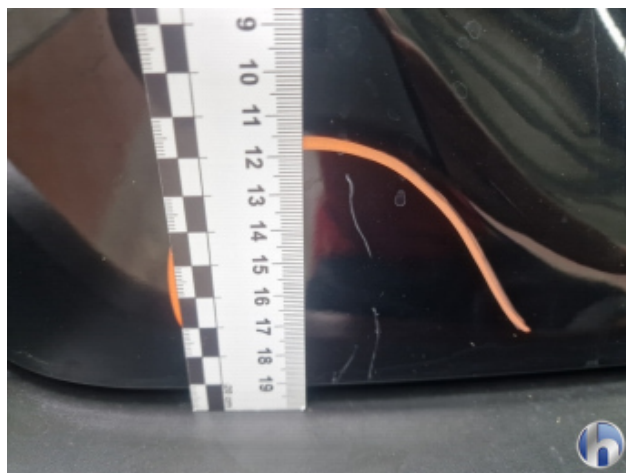
5. Heckklappe Kratzer - Smart Repair
