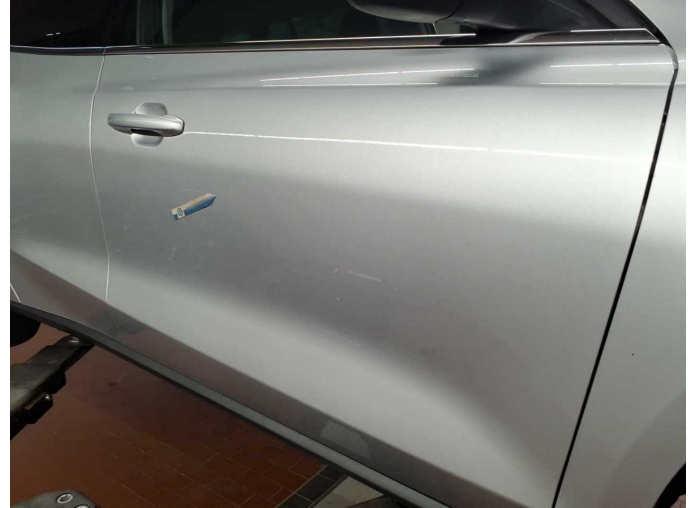
Damage 2: Door - front right side: Door - Scratch(es) - Smart repair
