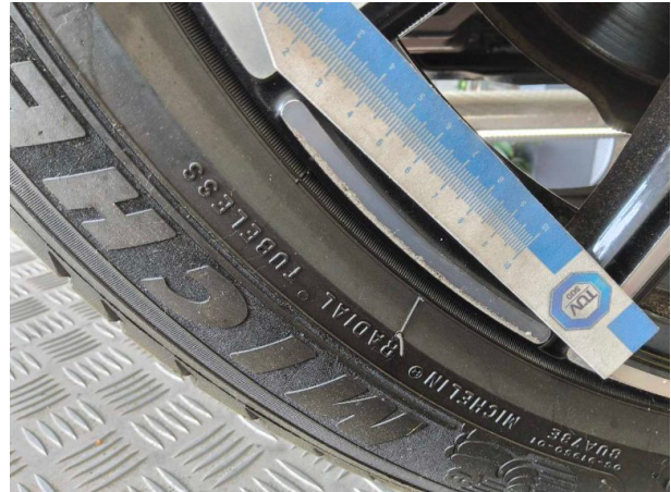
Damage #1: Wheel / tyres: Alloy rim - rear right side - Scratched - Loss in value
