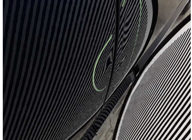
Damage #3: Door - rear right side: Door - dent(s) - Smooth repair work
