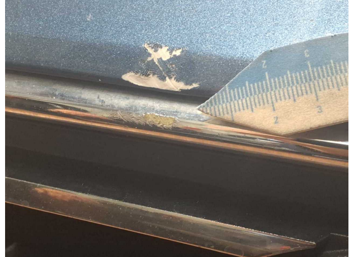
Damage 11: Front bumper: Front bumper (+ Kühlergrill verschärft erneuern) - Dent / paintcoat damage - Repair and paint
