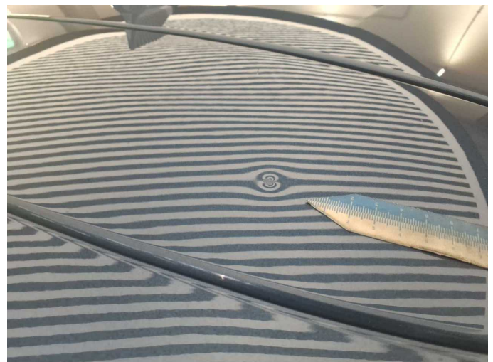
Damage 5: Boot lid / rear door: Boot lid - Dent / paintcoat damage - Smart repair
