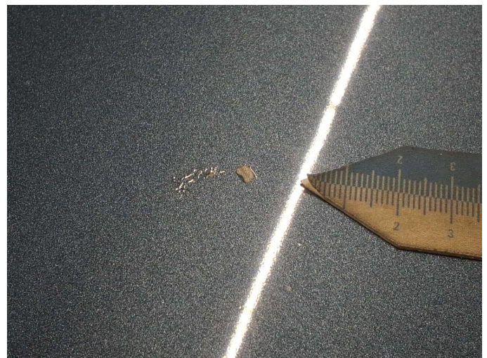
Damage 9: Bonnet: Bonnet - Paint defect - Paint
