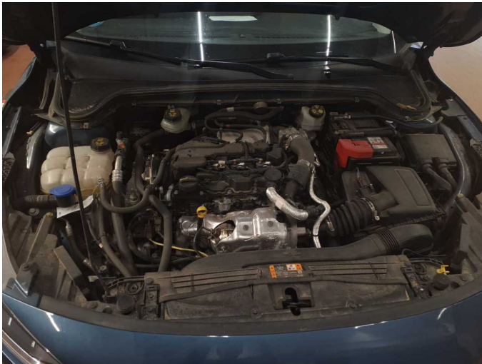
Missing part 1: Engine: Engine cover - Missing - Replace
