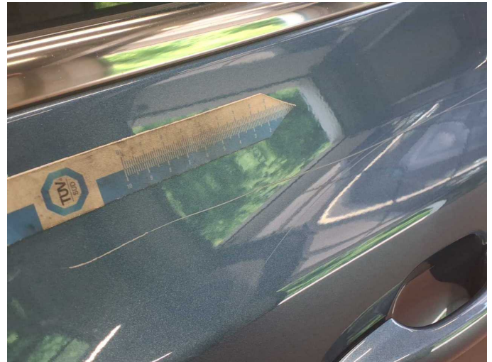
Damage 8: Door - rear left side: Door - Scratch(es) - Paint
