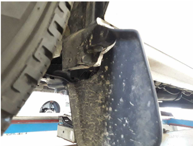
Damage 3: Mudguard - left side: Mud flap (Und rechts 2x) - Broken / torn - Replace
