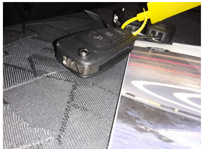
Damage 4: Equipment: Vehicle key with remote control (Schlüssel-bart fehlt) - Broken / torn - Replace
