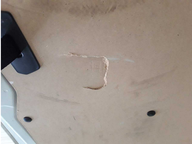
Damage 2: Boot lid / rear door: Trim plywood - lower - Broken / torn - Replace
