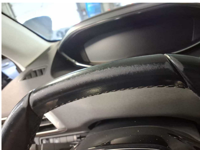
Damage 1: Steering system: Steering wheel - Abrasion - Smart repair
