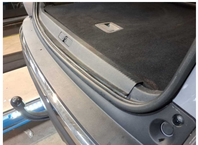
Damage 6: Trim / covers: Boot sill cover (Nasen gebrochen) - Loose - Replace
