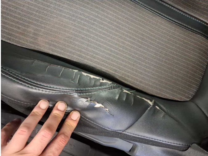
Damage 8: Seat - front: Seat cover - left side (Wange) - Broken / torn - Replace
