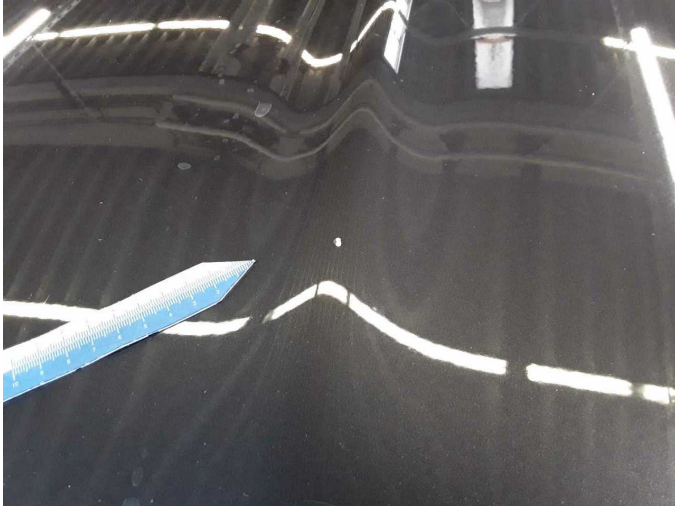
Damage 11: Bonnet: Bonnet - Stone chips - Paint
