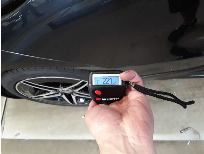
Repainting 1: Side panel - rear right side, Door - rear right side
