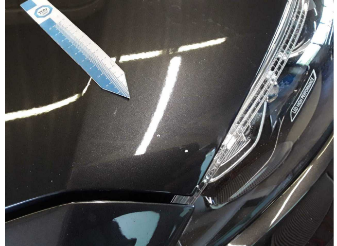
Damage 11: Bonnet: Bonnet - Stone chips - Paint
