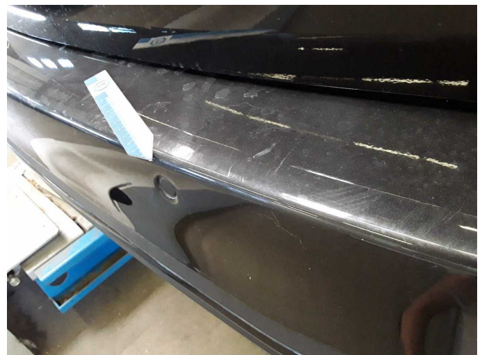
Damage 10: Rear bumper: Rear bumper - Scratched - Paint
