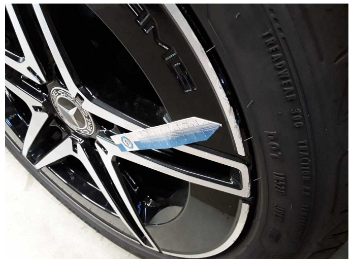
Damage 4: Wheel / tyres: Alloy rim - rear left side - Scratched - Loss in value
