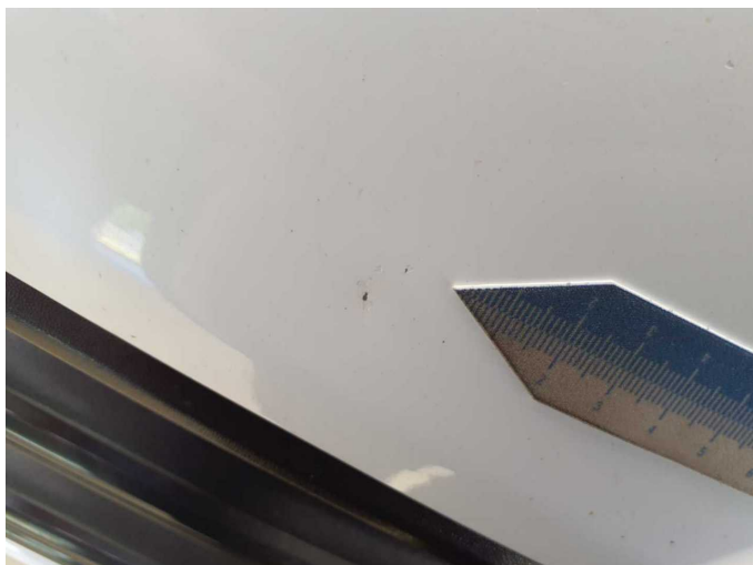
Damage 9: Bonnet: Bonnet - Dent / paintcoat damage - Paint
