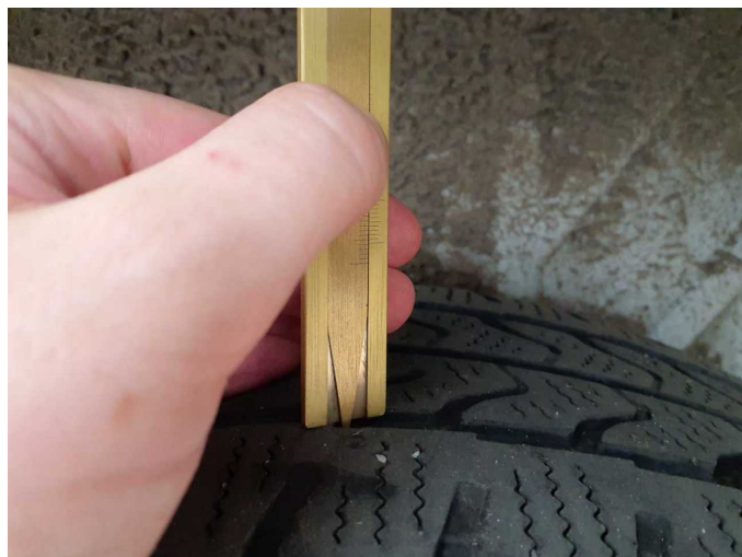
Wear and tear 5: Wheel / tyres: Tyre - rear right side (4,1mm) - Abrasion - No deduction
