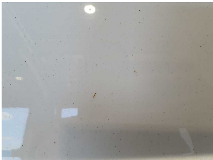
Damage 7: Body: Body - Stone chips - Conditioning
