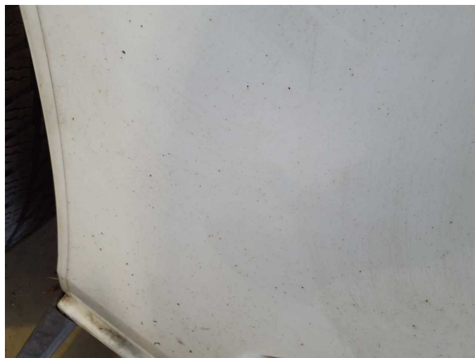
Damage 7: Body: Body - Stone chips - Conditioning
