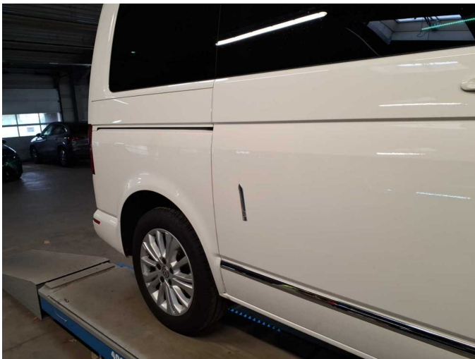
Damage 3: Sliding door, right: Sliding door with glass panel - dent(s) - Smooth repair work
