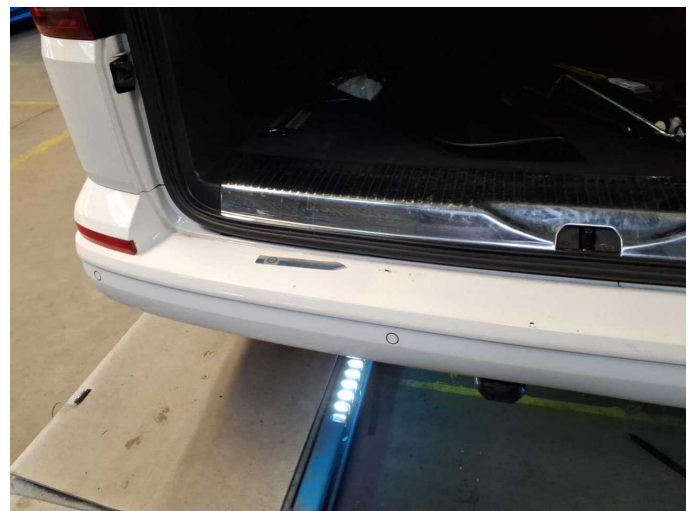
Damage 7: Rear bumper: Rear bumper - Scratch(es) - Paint
