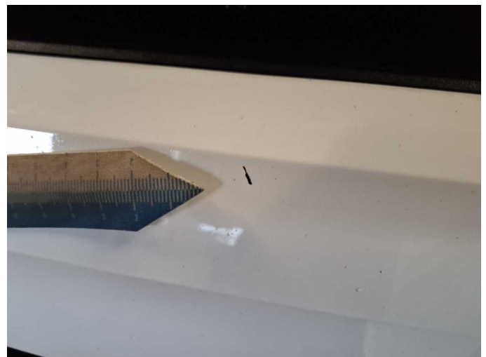
Damage 9: Front bumper: Front bumper (Steinschlag + Gitter V R erneuern) - Scratch(es) - Paint
