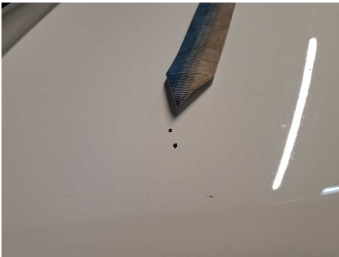
Damage 8: Bonnet: Bonnet - Stone chips - Paint
