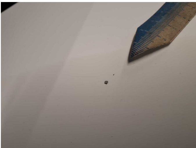
Damage 8: Bonnet: Bonnet - Stone chips - Paint
