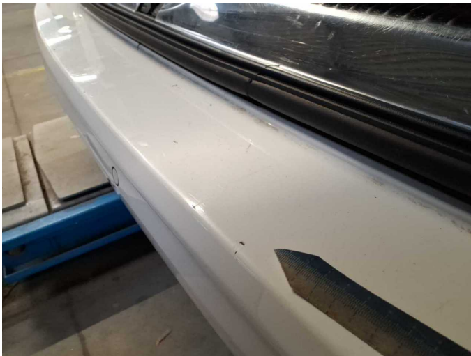
Damage 7: Rear bumper: Rear bumper - Scratch(es) - Paint
