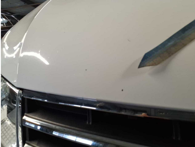
Damage 8: Bonnet: Bonnet - Stone chips - Paint
