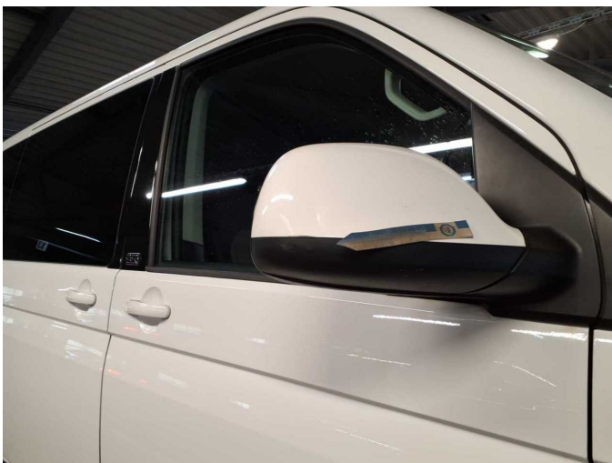
Damage 4: Wing mirror - right side: Mirror housing - Scratched - Replace
