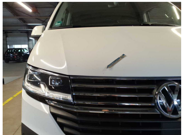
Damage 8: Bonnet: Bonnet - Stone chips - Paint
