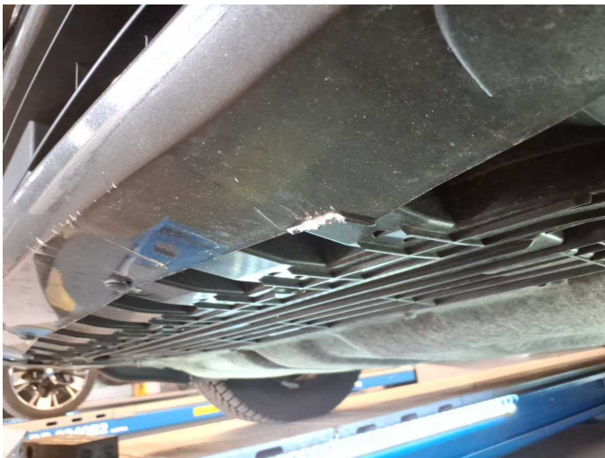
Damage 2: Front bumper: Spoiler - Scratch(es) - Smart repair
