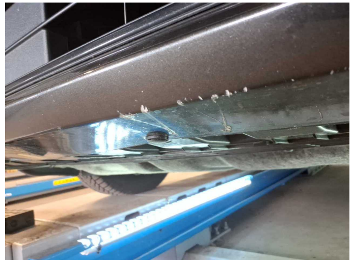
Damage 2: Front bumper: Spoiler - Scratch(es) - Smart repair
