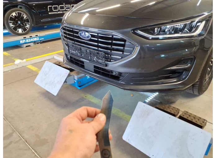
Damage 2: Front bumper: Spoiler - Scratch(es) - Smart repair
