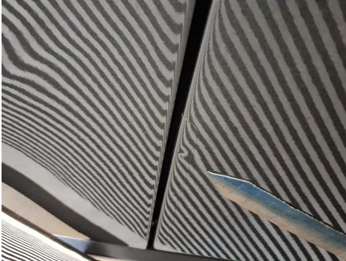
Damage 1: Side panel - rear left side: Side panel - dent(s) - Smooth repair work
