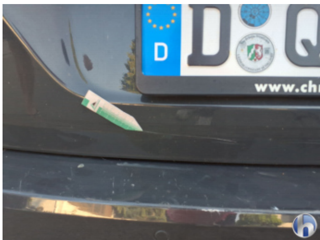
2. Heckklappe Kratzer - Smart Repair
