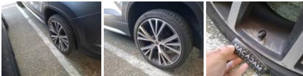
Tyre RL, Out of tolerance, Replace
