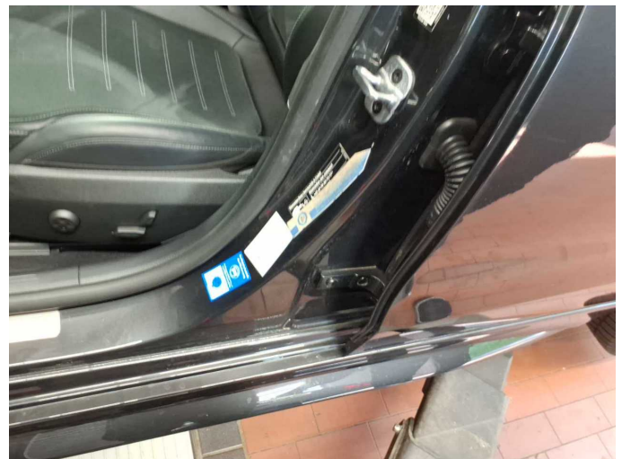
Damage 5: Sill - left side: Sill - Dent / paintcoat damage - Smart repair
