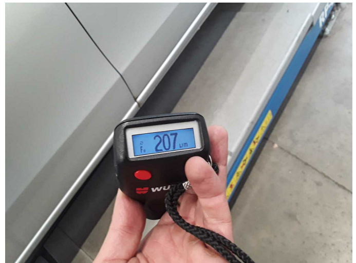
Repainting 1: Mudguard - right side, Side panel - rear right side, Door - front right side
