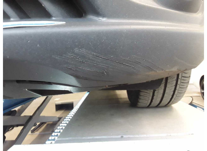
Wear and tear 1: Front bumper: Front bumper (unpainted) - Scratched - No deduction
