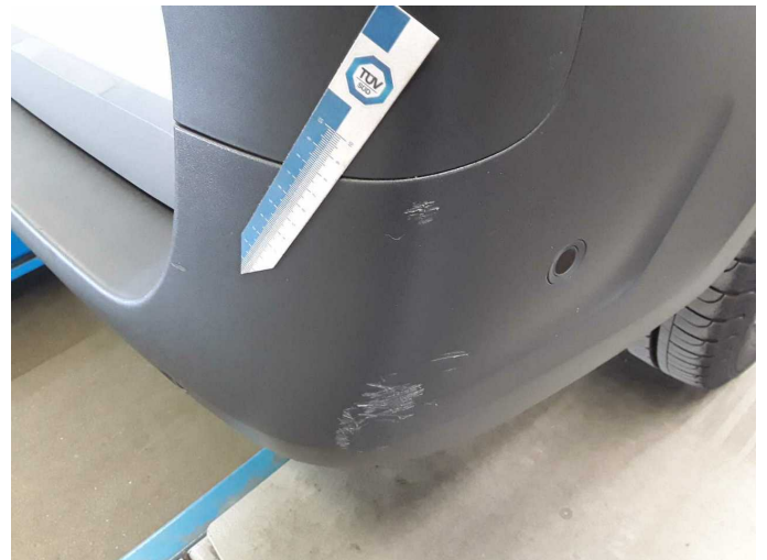
Wear and tear 2: Rear bumper: Rear bumper (unpainted) - Scratched - No deduction
