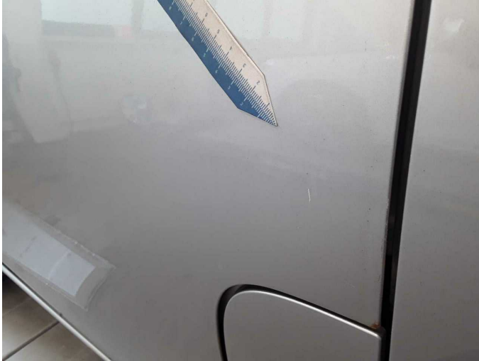
Wear and tear 4: Door - front left side: Door - Dent / paintcoat damage - No deduction
