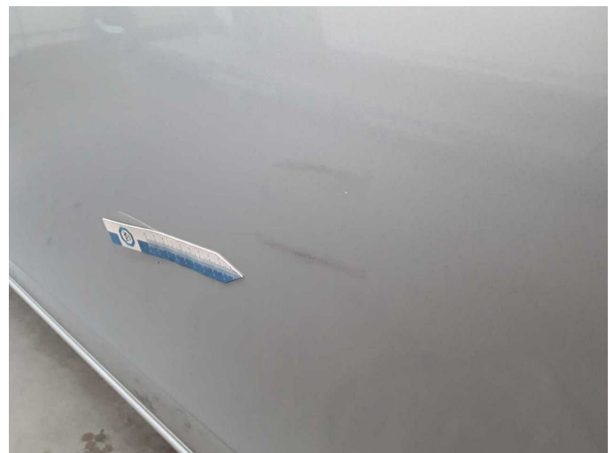
Damage 4: Sliding door - left side: Sliding door (Unterhalb nachlackiert) - Does not meet the leasing specifications - Paint
