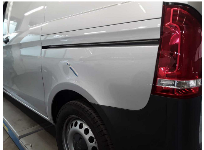
Damage 6: Side panel - rear left side: Side panel (Unterhalb nachlackiert) - Does not meet the leasing specifications - Paint
