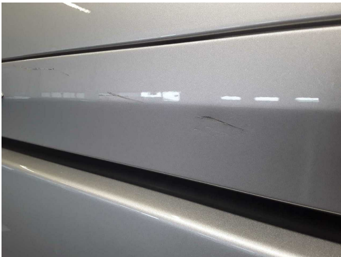
Damage 5: Side panel - rear right side: Side panel (Abdeckung) - Dent / paintcoat damage - Repair and paint
