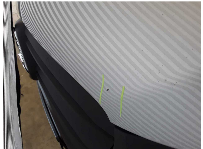
Damage 7: Bonnet: Bonnet - Dent / paintcoat damage - Repair and paint
