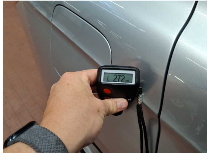
Repainting 2: Side panel - rear right side
