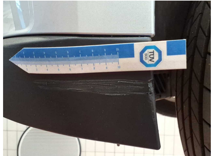
Damage 4: Front bumper: Spoiler - Scratched - Replace
