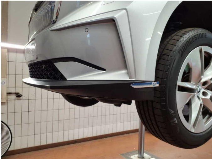
Damage 4: Front bumper: Spoiler - Scratched - Replace
