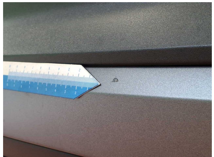
Damage 3: Rear bumper: Spoiler - Scratch(es) - Smart repair
