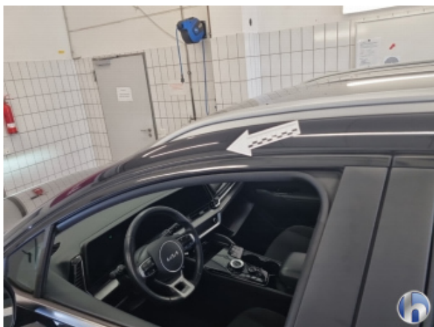
1. Dachrahmen - Links 1 Delle - Sanft Instandsetzen
