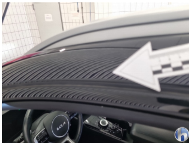
1. Dachrahmen - Links 1 Delle - Sanft Instandsetzen
