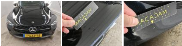
Windscreen, Stone chip(s), Windscreen repair
