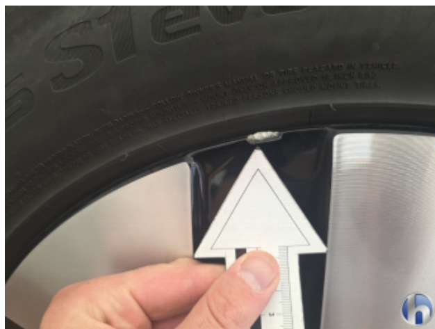
5. Felge Vorne - Links Kratzer - Smart Repair
