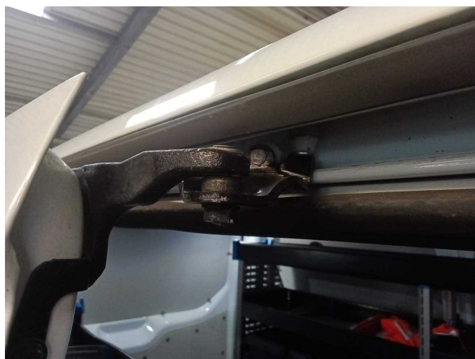
Damage 3: Sliding door, right: Sliding door - Malposition - Set / adjust
