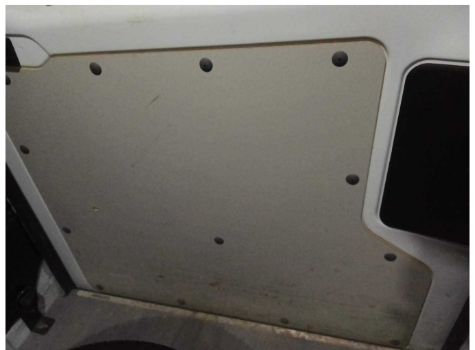
Damage 2: Trim / covers: Door trim - rear right side - Holes - Replace
