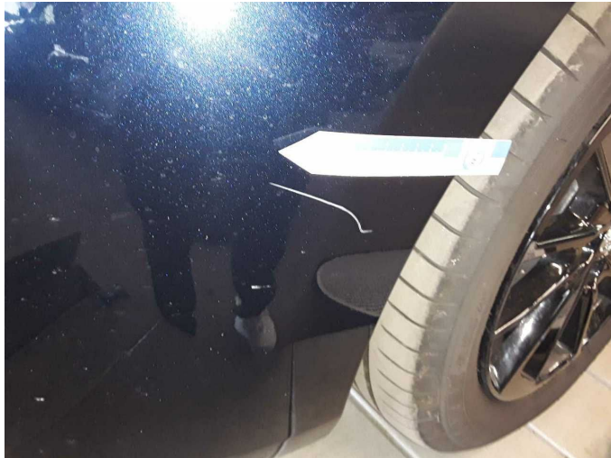
Damage 5: Front bumper: Front bumper - Scratch(es) - Paint
