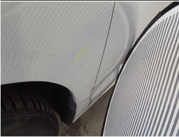
Damage #9: Mudguard - left side: Mudguard - left side - dent(s) - Repair and paint
