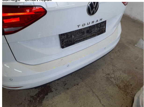
Damage #6: Rear bumper: Rear bumper - Scratched - Smart repair
