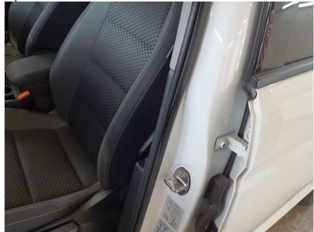
Damage #3: Door - front left side: Door seal - Porous / cracked - Replace
