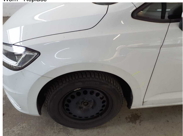
Damage #9: Mudguard - left side: Mudguard - left side - dent(...) - Repair and paint
