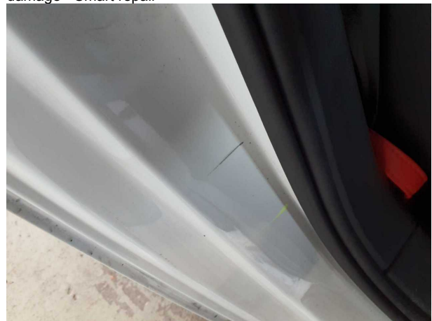
Damage #5: Side panel - rear right side: Sill - Dent / paintcoat damage - Smart repair
