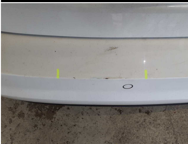
Damage #6: Rear bumper: Rear bumper - Scratched - Smart repair
