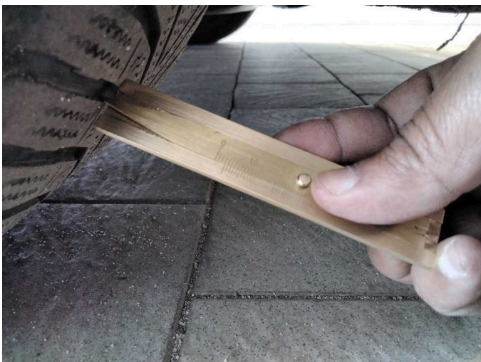
Damage 3: Wheel / tyres: Tyres - complete set (3mm bis 4mm) - Does not meet the leasing specifications - Replace
