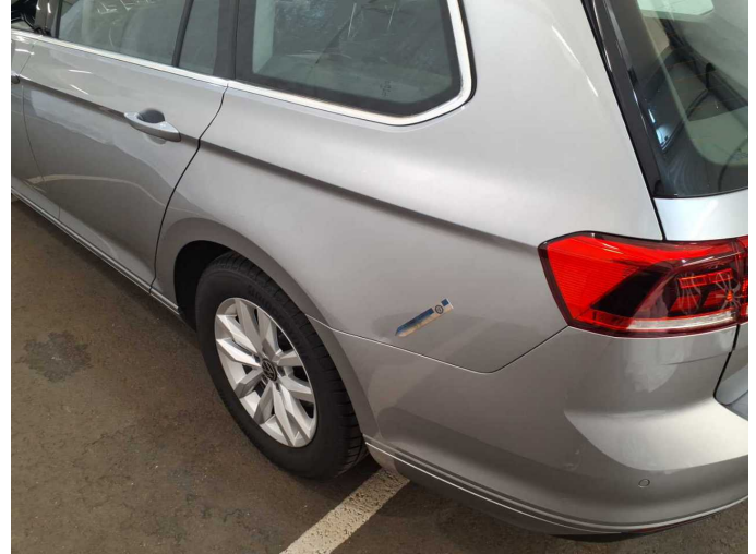
Damage 4: Side panel - rear left side: Side panel - Dent / paintcoat damage - Repair and paint
