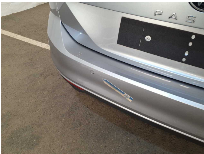
Damage 2: Rear bumper: Rear bumper - Scratch(es) - Paint
