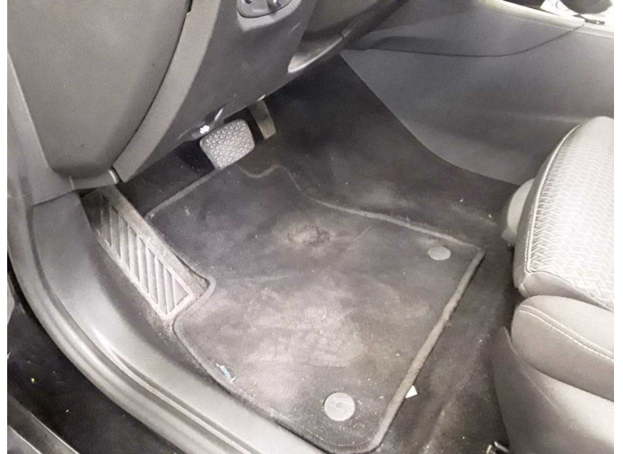
Damage 2: Trim / covers: Floor mats - Damaged - Replace
