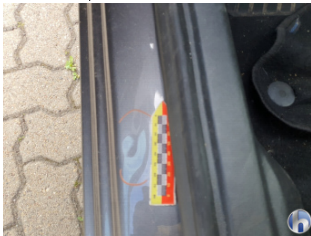
2. Türeinstieg Vorne - Links 1 Delle - Smart Repair
