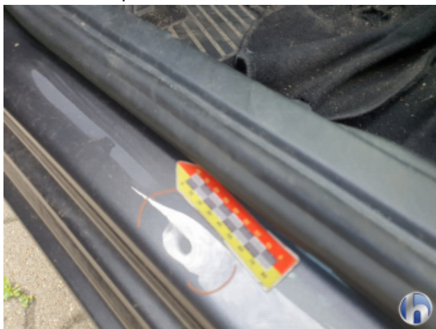
2. Türeinstieg Vorne - Links 1 Delle - Smart Repair
