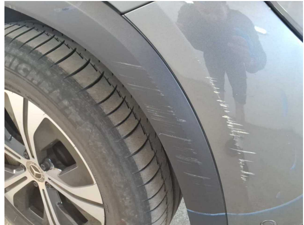
Damage #3: Mudguard - right side: Wheel well extension - Scratched - Replace
