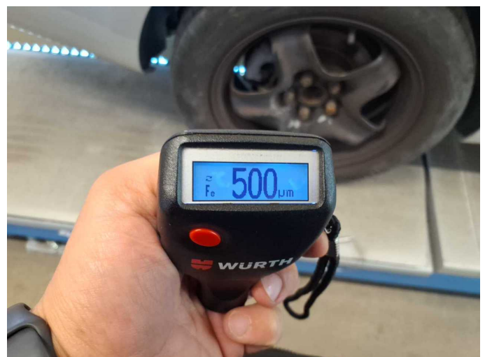
Repainting 1: Boot lid / rear door, Bonnet, Side panel - rear left side, Side panel - rear right side
