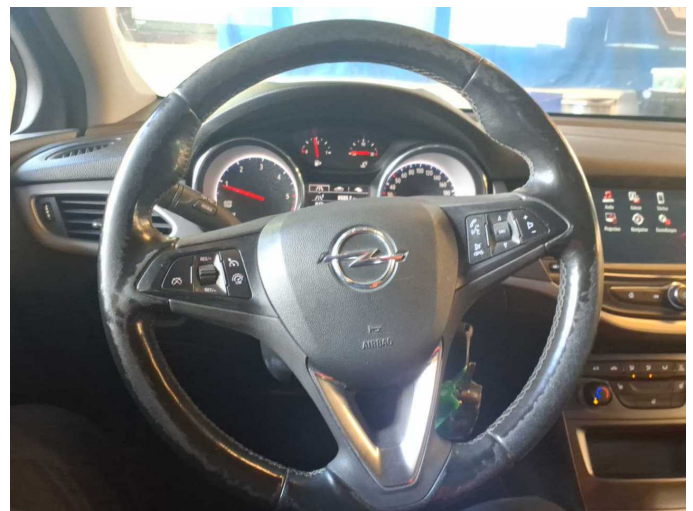
Wear and tear 1: Steering system: Steering wheel sheath - Scratched - No deduction
