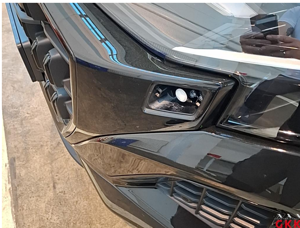
Picture 21 headlight cleaning system, cover, missing, replace
