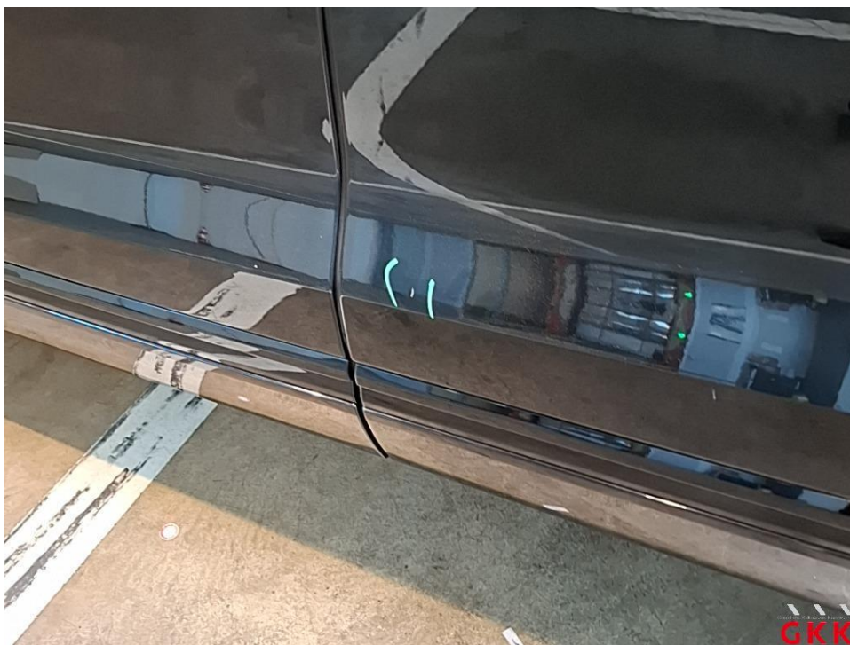
Picture 19 door rear left, scratched, disassemble, grind, polish
