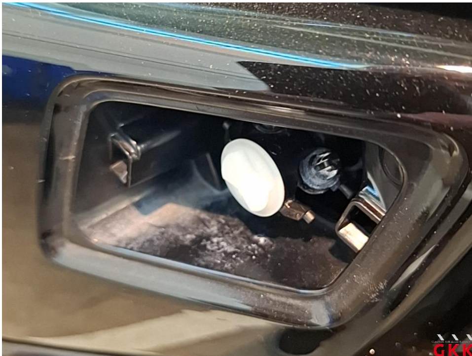
Picture 22 headlight cleaning system, cover, missing, replace
