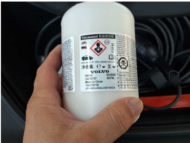
Damage #2: Equipment: Tirefit filler - Expired - Replace
