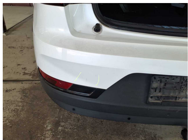
Damage #8: Rear bumper: Rear bumper - Scratched - Paint
