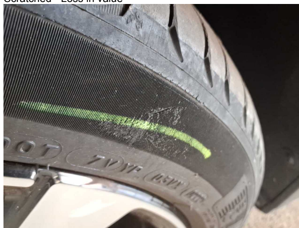
Damage #6: Wheel / tyres: Tyre - front left side - Damaged - Replace
