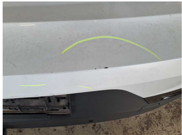
Damage #8: Rear bumper: Rear bumper - Scratched - Paint
