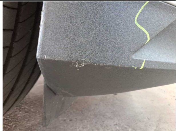
Damage #7: Front bumper: Spoiler - Scratched - Loss in value
