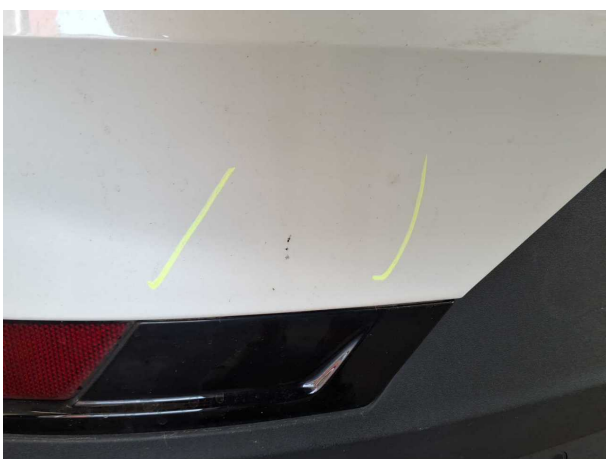
Damage #8: Rear bumper: Rear bumper - Scratched - Paint
