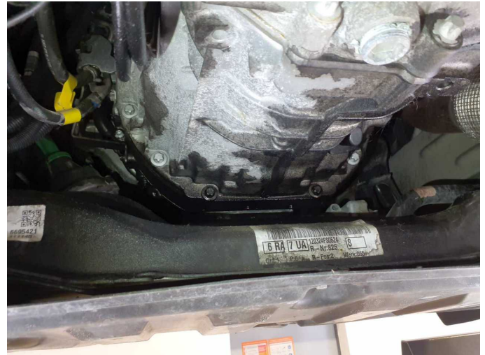
Damage 3: Gearbox: Gearbox - Leaking - Perform diagnosis
