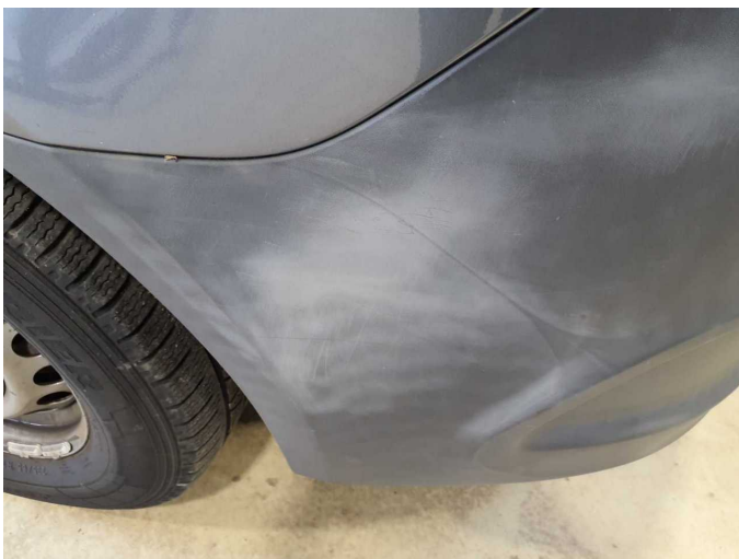
Damage 12: Front bumper: Front bumper - Worn - Loss in value
