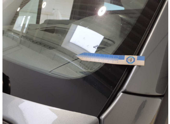
Damage 17: Vehicle glazing: Windscreen - Stone chips - repair according to calculation
