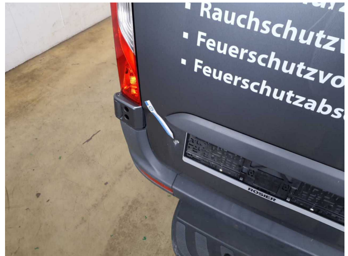
Damage 18: Boot lid / rear door: Rear door - left side - Broken / torn - repair according to calculation
