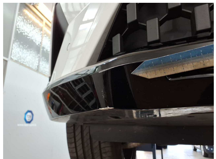
Damage 2: Front bumper: Spoiler - Scratch(es) - Smart repair
