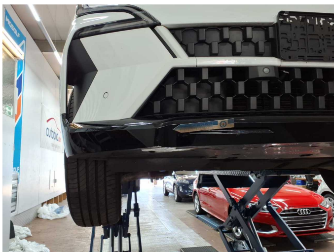
Damage 2: Front bumper: Spoiler - Scratch(es) - Smart repair
