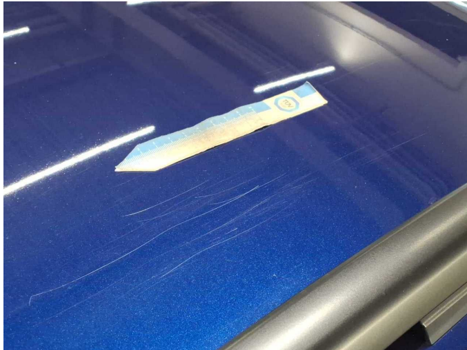
Damage 4: Roof: Roof - Scratch(es) - Paint
