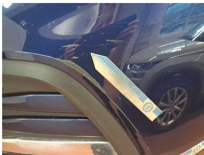
Damage 3: Front bumper: Front bumper - Scratched - Paint
