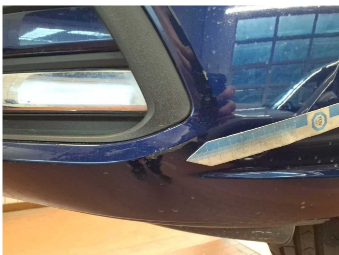
Damage 3: Front bumper: Front bumper - Scratched - Paint
