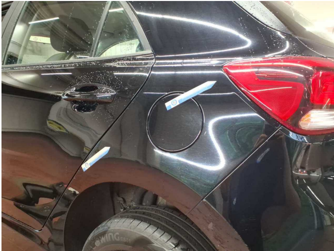
Wear and tear 5: Side panel - rear left side: Side panel - Scratch(es) - No deduction
