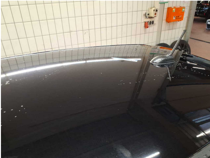
Damage 14: Roof: Roof - Scratch(es) - Paint
