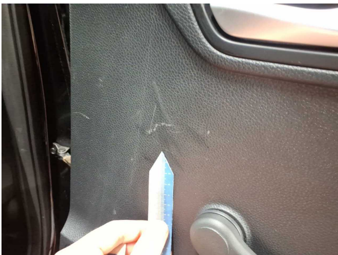
Wear and tear 4: Trim / covers: Door trim - rear right side - Scratch(es) - No deduction
