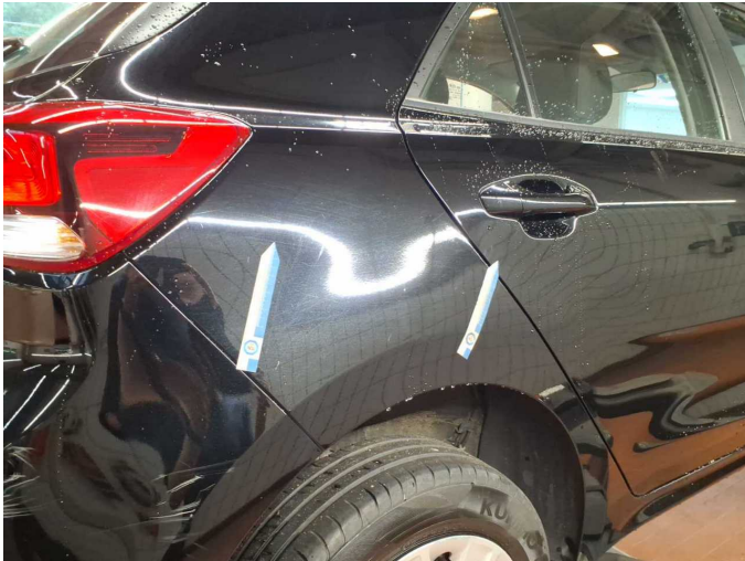
Damage 7: Side panel - rear right side: Side panel - Scratch(es) - Smart repair
