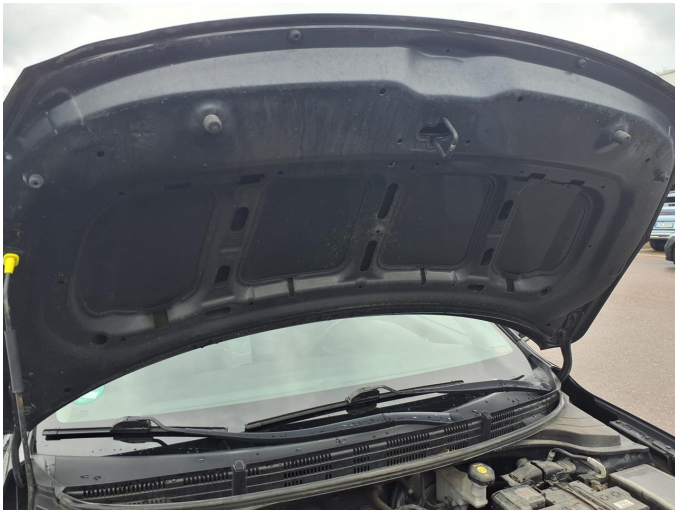
Damage 10: Bonnet: Insulation lining - Missing - Replace
