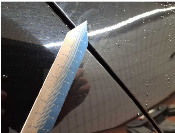
Damage 7: Side panel - rear right side: Side panel - Scratch(es) - Smart repair
