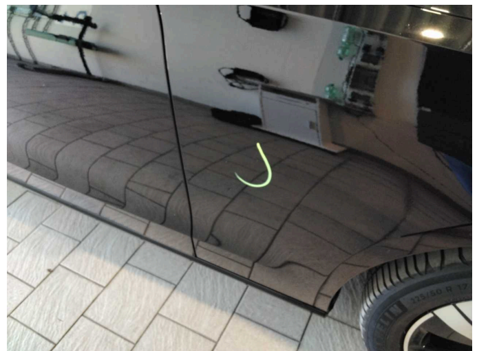
Wear and tear 4: Mudguard - right side: Mudguard - right side - Dent / paintcoat damage - Smart repair
