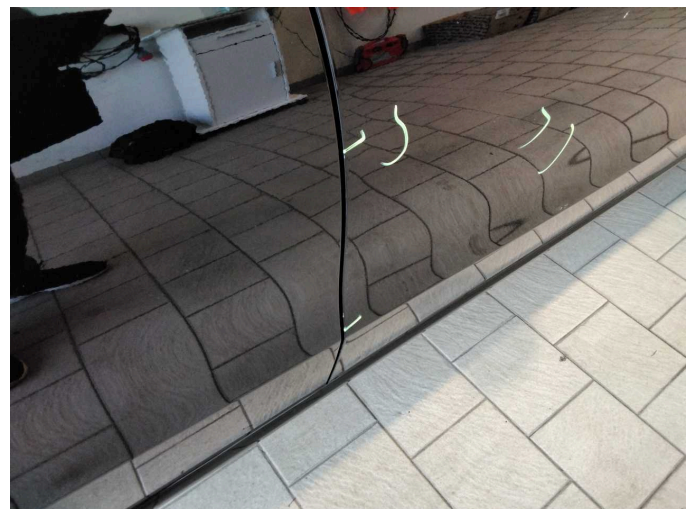
Wear and tear 9: Door - front right side: Door edge - Scratch(es) - Smart repair
