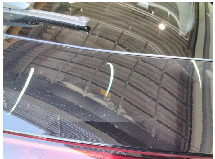
Damage 7: Boot lid / rear door: Boot lid - Scratch(es) - Paint
