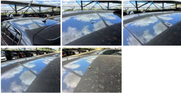
Roof, Hail damage, Repair and paint (complete)
