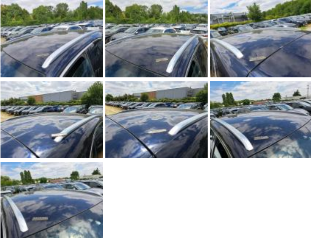
Roof, Hail damage, Repair and paint (complete)
