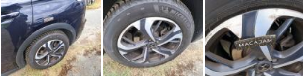
Tyre FR, Out of tolerance, Replace
