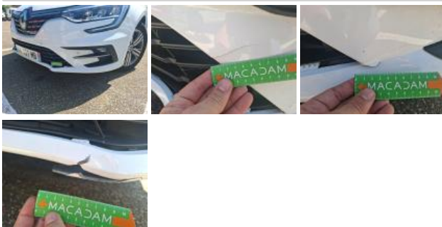
Bumper grille, Broken, Replace
