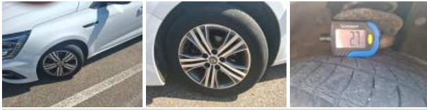
Tyre FR, Out of tolerance, Replace
