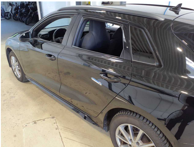
Damage 3: Door - rear left side: Door - dent(s) - Smart repair
