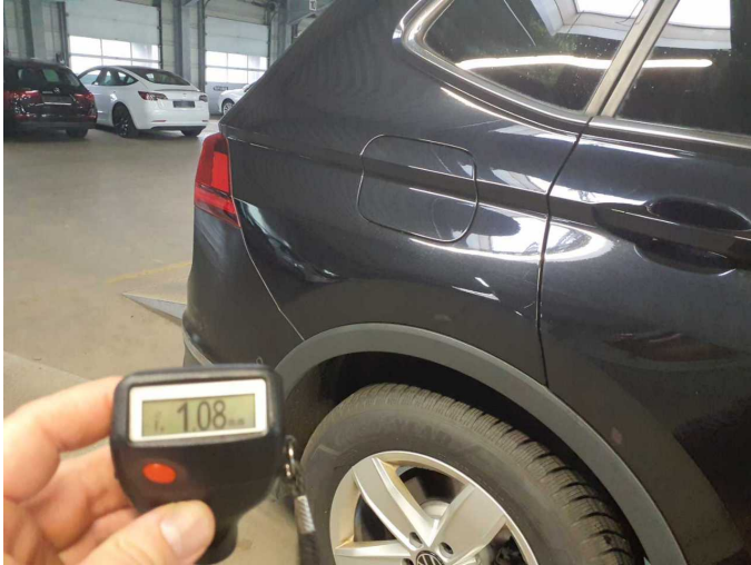
Repainting 2: Side panel - rear right side
