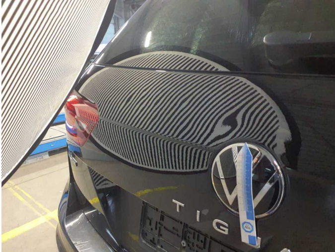
Damage 5: Boot lid / rear door: Boot lid - Deformed - Repair and paint
