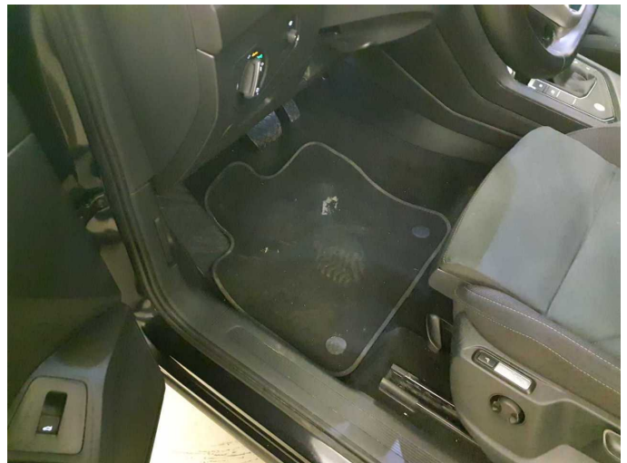
Damage 1: Trim / covers: Floor mats - Holes - Replace
