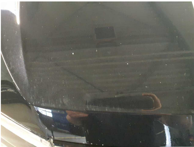
Damage 7: Bonnet: Bonnet - Stone chips - Paint
