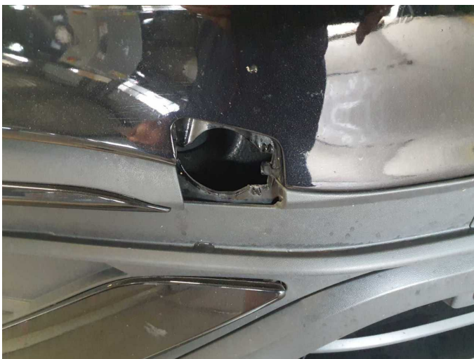
Missing part 1: Equipment: Towing eye (Abdeckung) - Missing - Replace
