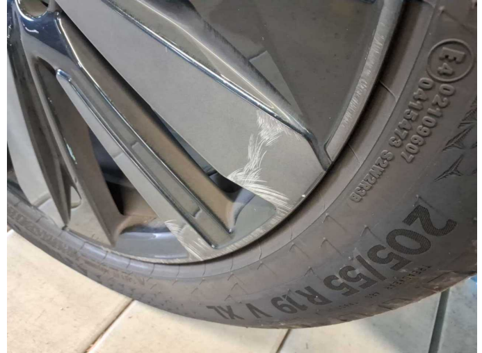
Damage 8: Wheel / tyres: Alloy rim - front left side - Scratched - Loss in value
