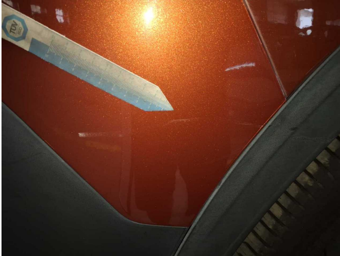
Damage 11: Rear bumper: Bumper - rear right side - Scratched - Paint
