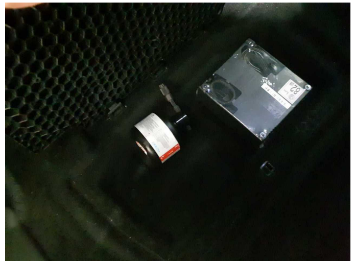
Damage 1: Equipment: Tirefit filler - Expired - Replace
