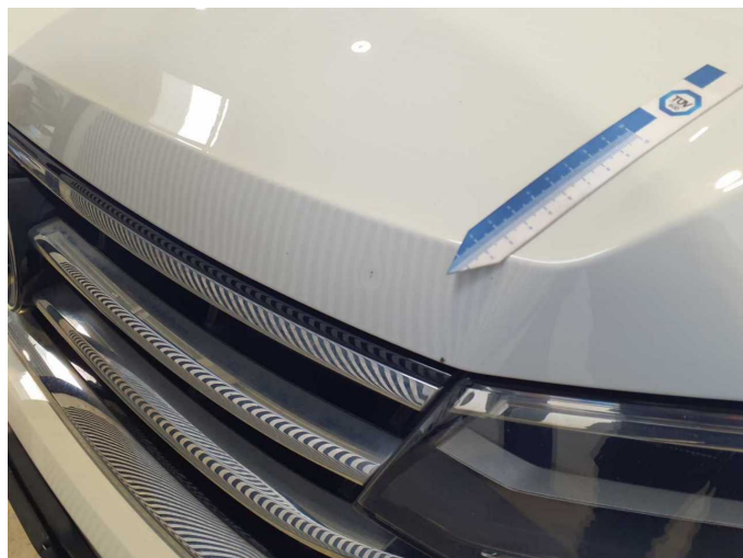
Damage 9: Bonnet: Bonnet (Korrosion) - Dent / paintcoat damage - Repair and paint
