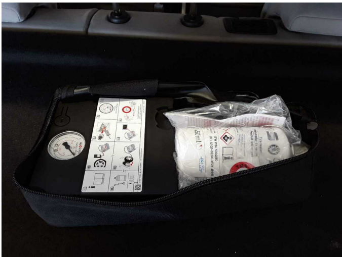
Damage 1: Equipment: Tirefit filler - Expired - Replace
