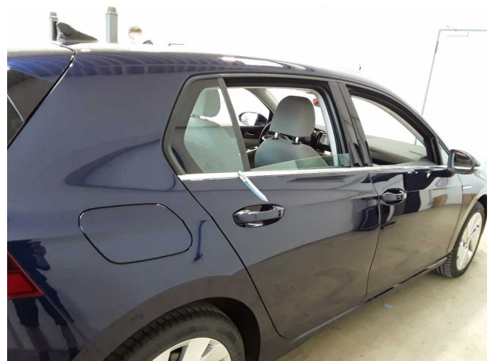
Damage 3: Door - rear right side: Door - Scratch(es) - Smart repair
