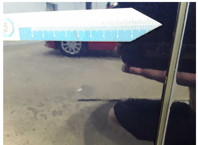
Damage 7: Door - front left side: Door (Einschlüsse) - Paint defect - Repair and paint
