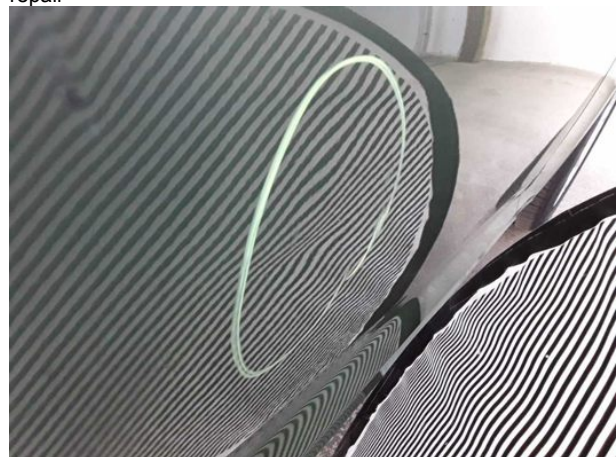
Damage #10: Door - front right side: Door - dent(s) - Smooth repair work
