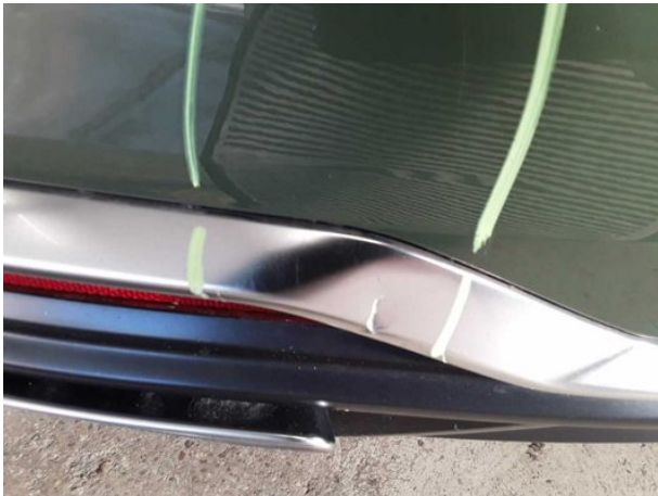
Damage #11: Rear bumper: Spoiler - Broken / torn - Replace
