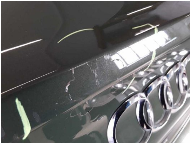
Damage #8: Boot lid / rear door: Boot lid - Scratched - Smart repair
