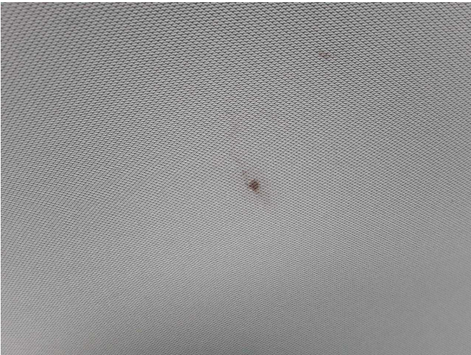
Damage 3: Trim / covers: Roof lining - Soiled - Clean
