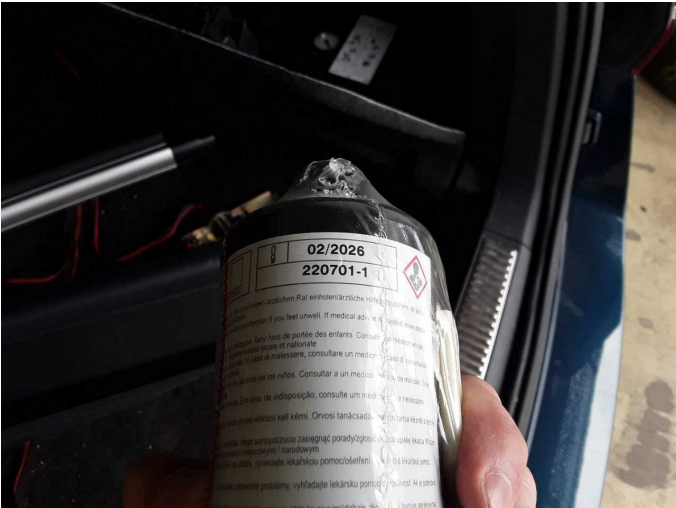
Damage 2: Equipment: Tirefit filler - Expired - Replace
