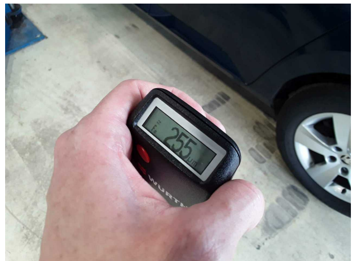
Repainting 1: Door - rear left side
