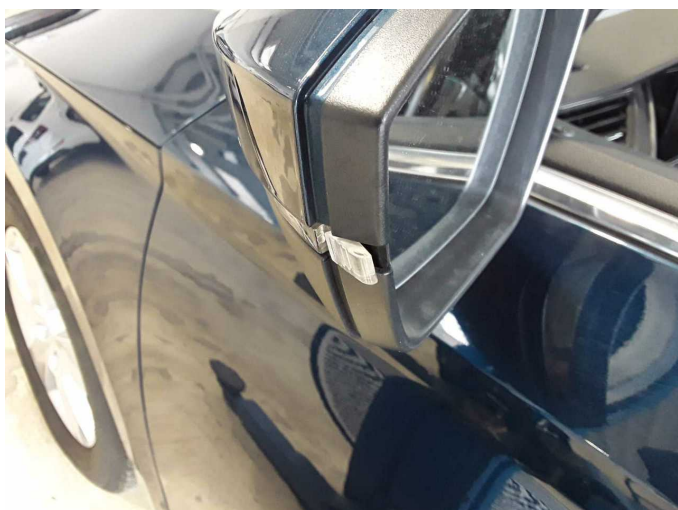
Damage 8: Indicator - front: Mirror - left side - Broken / torn - Replace
