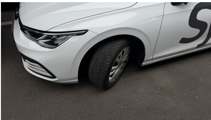
Damage 4: Wheel / tyres: Tyre - front left side (Profiltiefe 3mm + Ausbrüche in der Lauffläche) - Does not meet the leasing specifications - Replace
