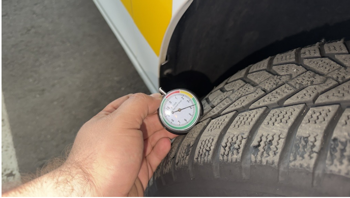
Damage 3: Wheel / tyres: Tyre - front right side (Profiltiefe 3mm + Ausbrüche in der Lauffläche) - Does not meet the leasing specifications - Replace
