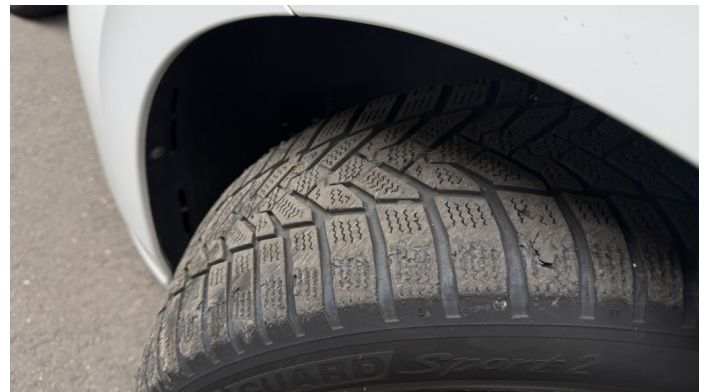
Damage 4: Wheel / tyres: Tyre - front left side (Profiltiefe 3mm + Ausbrüche in der Lauffläche) - Does not meet the leasing specifications - Replace
