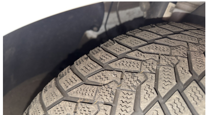
Damage 3: Wheel / tyres: Tyre - front right side (Profiltiefe 3mm + Ausbrüche in der Lauffläche) - Does not meet the leasing specifications - Replace
