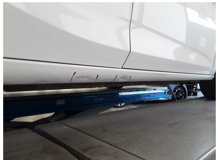
Damage 6: Sill - right side: Sill - dent(s) - Repair and paint
