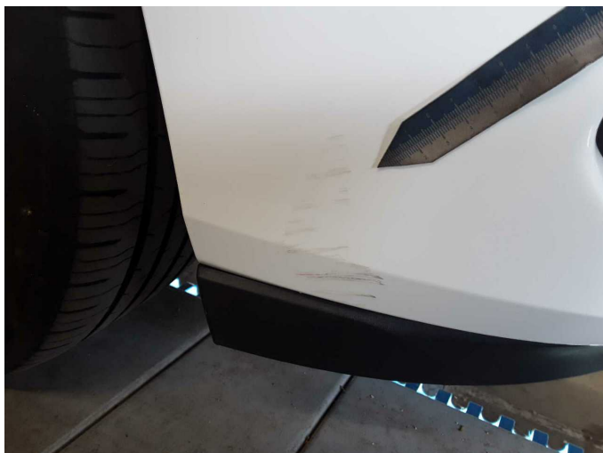
Damage 9: Front bumper: Front bumper (Inklusive Steinschläge) - Scratched - Paint
