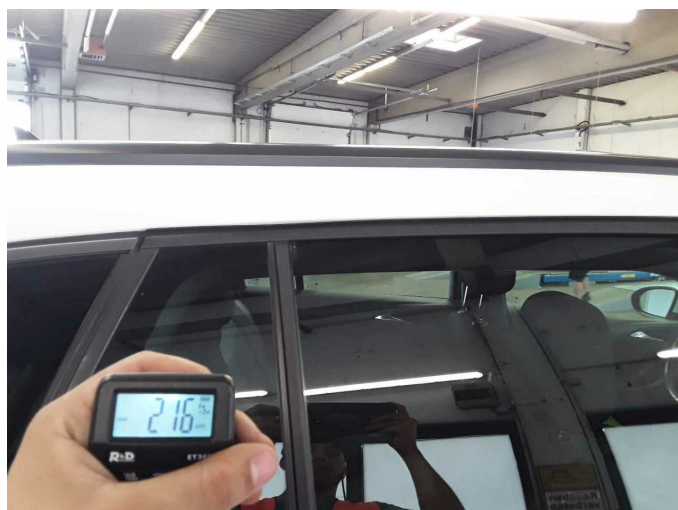
Roof rail - right side: 216 µm
