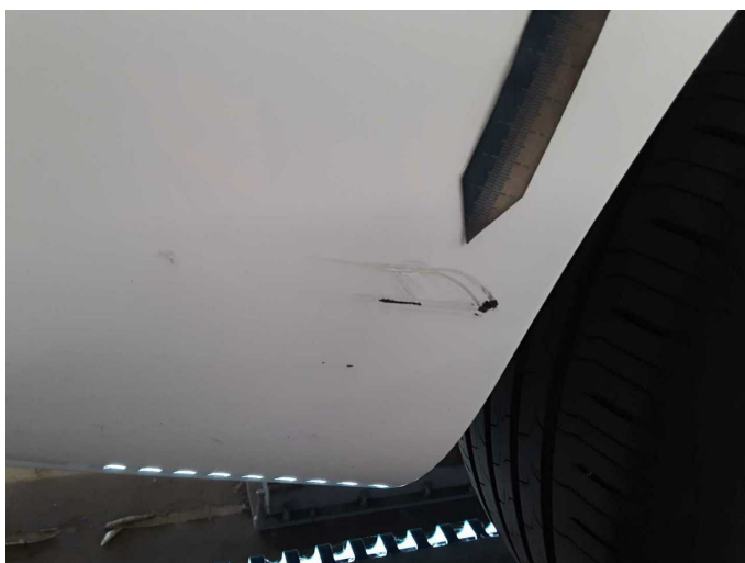
Damage 8: Rear bumper: Rear bumper - Scratched - Paint
